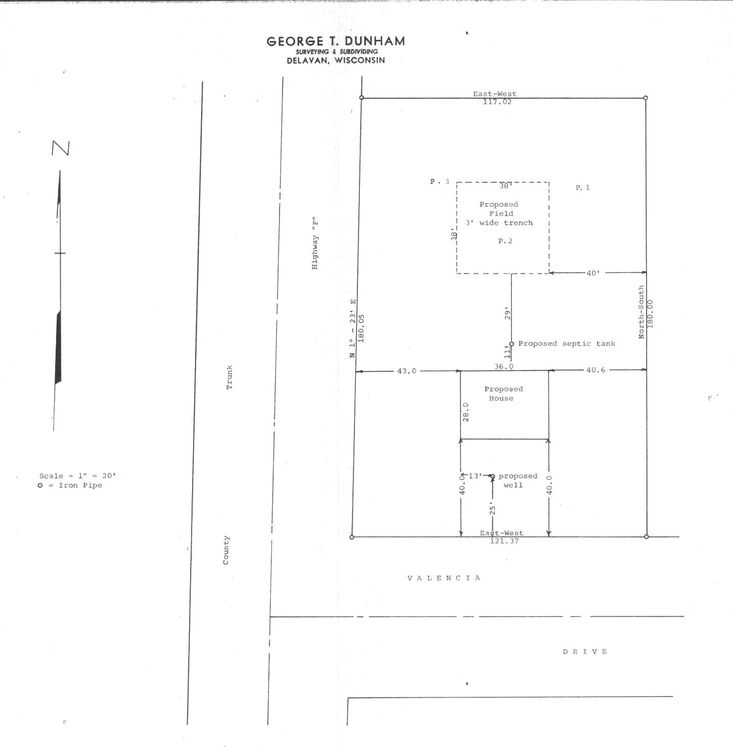
Plat of survey of Lot 1, Block 14 of Inlet Oaks Subdivision No. 5 located in Section 15, T 2 N, R 16 E, Walworth County, Wisconsin. Plat also shows the location of the percolation tests made on said lot and the location of the house to be built and of the well and drainage field to be placed on said lot. September 18, 1969
